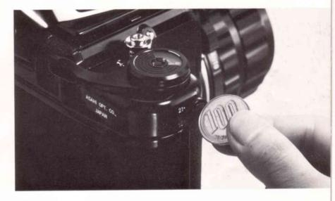
The film type dial (4) should also be properly set. Set it at 120 (indicated in green) for 120 roll-film, and at 220 (indicated in orange) for 220 roll-film.
