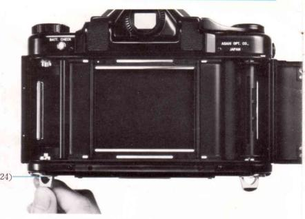
Pull down on the back cover release lever (20) to open the camera. The film spool retainer knobs (24) hold the film spools securely in place. To load or remove film, unfold the crank of the knob, turn it to the left until it stops, and pull out the knob.
