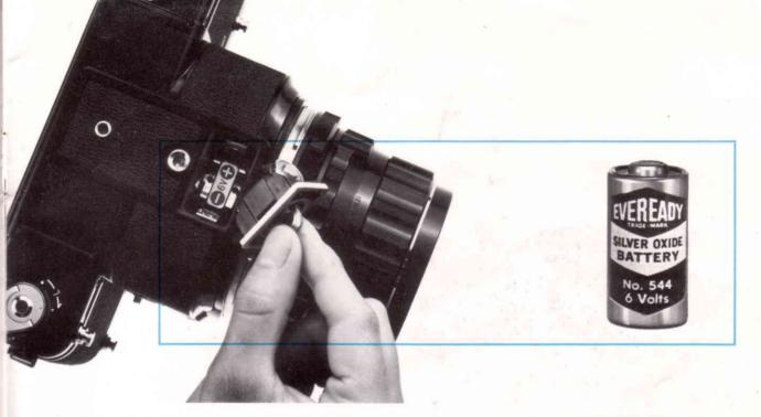
The silver oxide battery used in your camera will last for about  $8,000 \sim 10,000$  exposures. To check the battery condition, depress the battery check button (21); the red battery check lamp (14) will glow if the battery is still in good condition.
