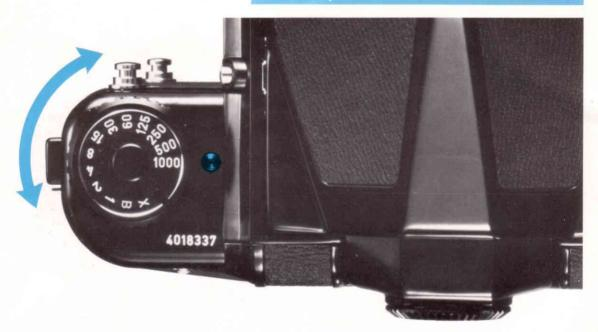
The click-stopped shutter speed dial is actually a rotary electrical switch that brings a series of individual precision wire-wound resistors into play for each shutter speed. Because of this, intermediate speeds cannot be set. The shutter release button accepts a conventional cable release.
